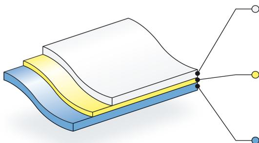
**Facestock:** 2 mil optically clear scratch resistant topcoated polyester that offers excellent clarity and dimensional stability combined with good high temperature and humidity resistance. The optically clear polyester provides high resolution imaging with excellent adhesion to UV curable inks.
