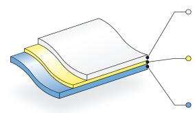
**Facestock:** 2 mil optically clear topcoated polyester that offers excellent clarity and dimensional stability combined with good high temperature and humidity resistance. The optically clear polyester provides high resolution imaging with excellent adhesion to UV curable inks.
